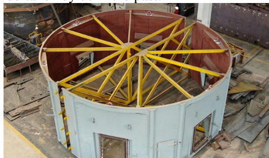
TYPE O– JOB - Mill Housing Industry – Cement Plant HEIGHT AND Width –4.5 meter Height and 10 meter Dia241 approx. approx. W–IGHT - –5241 approx. approx
