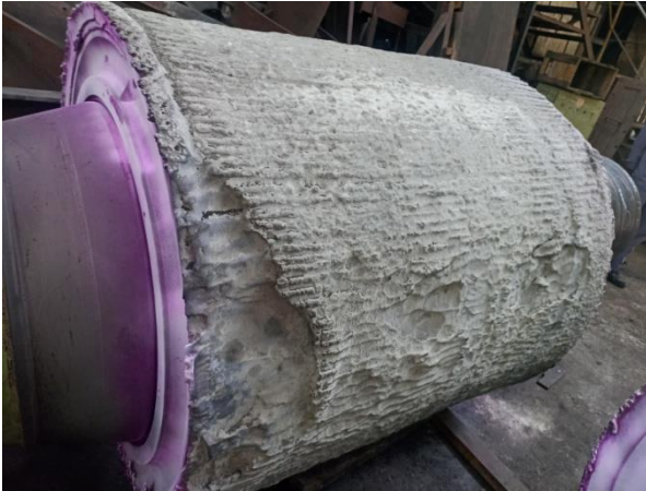
Roller Press–Roll - Worn out
