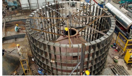
TYPE O– JOB - Separator Rotor Industry – Cement Plant HEIGHT AND Width –4.5 Meter and 6 Meter Diameter W–IGHT - 242pprox.approx
