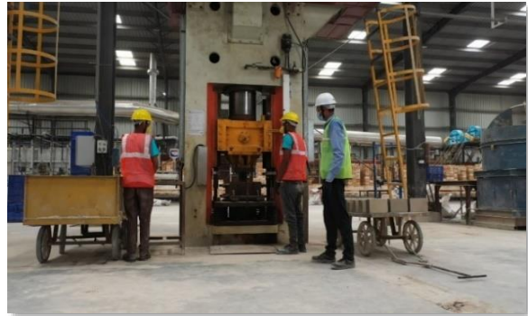
Press machine for making the bricks
