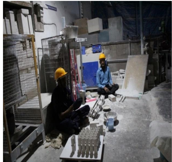
Slipcasting area-ferrule making- slip casting method is pouring of the raw material into moulds for making tubes such as ferrule
