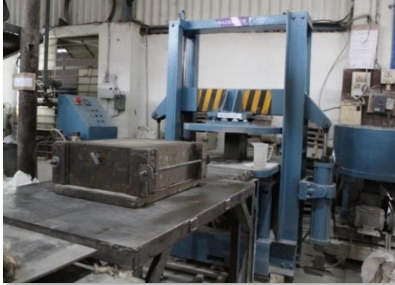
Maxibrator-for complicated production- intricate shapes of any size are made using our maxibrator machine wherein the mould is pressed in the maxibrator machine
