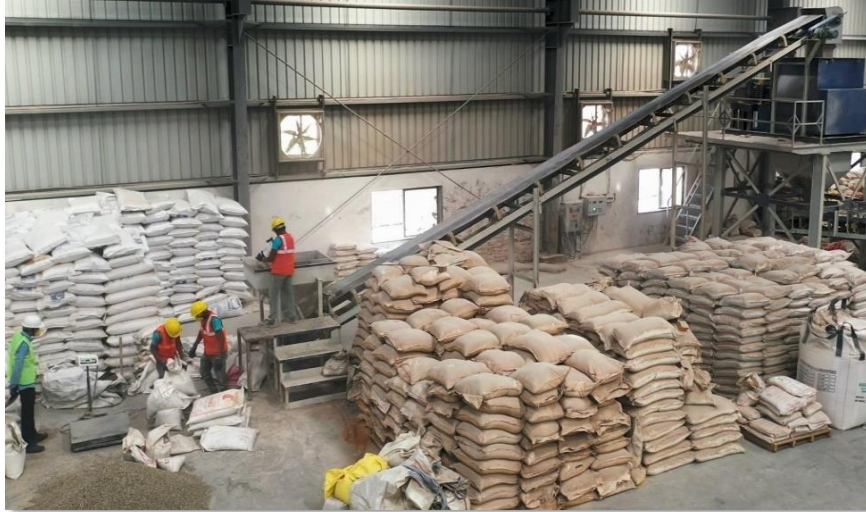
Mixing and packing of Castable
