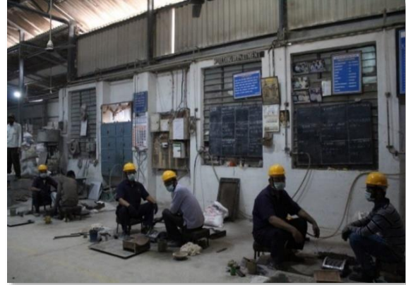
Moulding department – the moulds are checked for the dimension prior to sending for production. Intricate shaped bricks are hand moulded.
