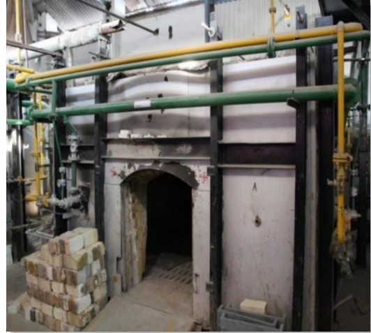
Kiln –A (4ton) – natural gas fired downdraft kiln for firing the material
