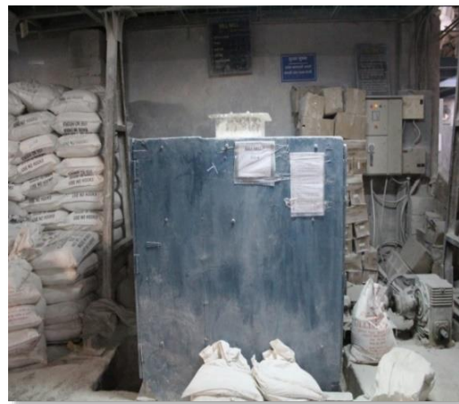
Ball mill-2 – for crushing raw material into fine powder
