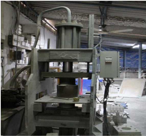
Hydraulic press (50 ton)-for small product making– small size bricks are pressed in our hydraulic press of 50 ton capacity
