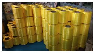
PP Multifilament yarn refers to a type of yarn made from polypropylene (PP) fibers that are extruded into multiple filaments and then twisted or spun together to form a single strand. Polypropylene is a thermoplastic polymer known for its excellent strength, durability, and resistance to chemicals, moisture, and UV radiation.
