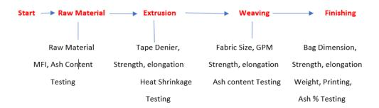
**Raw Material Testing**: - Poly Propylene Melt Flow Index testing and CaCo3 % in Polypropylene and Filler Masterbatch.
