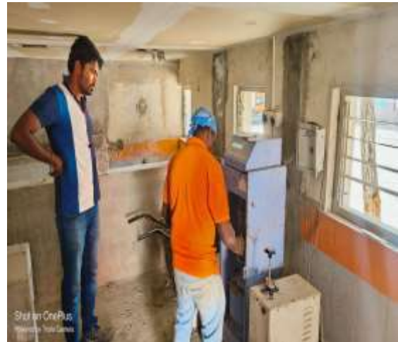
PCC Concrete Trial Mix Testing
