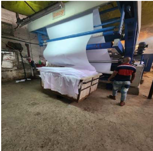
Jiger Machine For Dying over the fabrics
